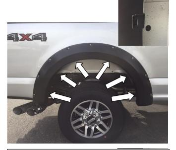
**STEP 11:** Place the Fender Flare onto the vehicle and fit into the correct position following the contours of the body. Use six (6) provided "U" Shaped Retention Clips to secure the Fender Flare to the body. Ensure the barb in the clip securely attaches in the slot on the Fender Flare. REPEAT ALL ABOVE STEPS FOR OPPOSITE SIDE OF VEHICLE.
