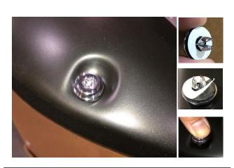
**STEP 8:** Attach the extruded plastic bolts. Peel back white tape liner from the bottom side of the extruded plastic bolt and press until it snaps into place. Ensure inside of Fender Flares where the rubber seal is attached is clean, using the alcohol wipes provided. Wipe away any residue with a dry clean cloth.
