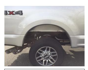
**STEP 10:** Clean the body areas where the Fender Flares will makes contact. A light misting on fender using a soap and water solution can aid in proper rubber placement.
