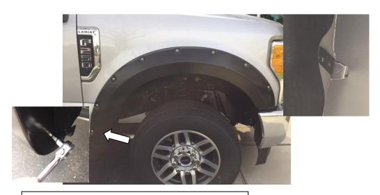
**STEP 7:** Loosely reinstall the lowest rear 7/32" socket head screws through slot in the Fender Flare to the vehicle. Make sure the screws are securely engaged to the vehicle fender. Install provided Long Attachment Clips in remaining four (4) Fender Flare Slots. Loosely reinstall remaining 7/32 in socket head screws. Ensure part is still in the position of best fit and extrusion is in correct position before hand tightening all screws.
